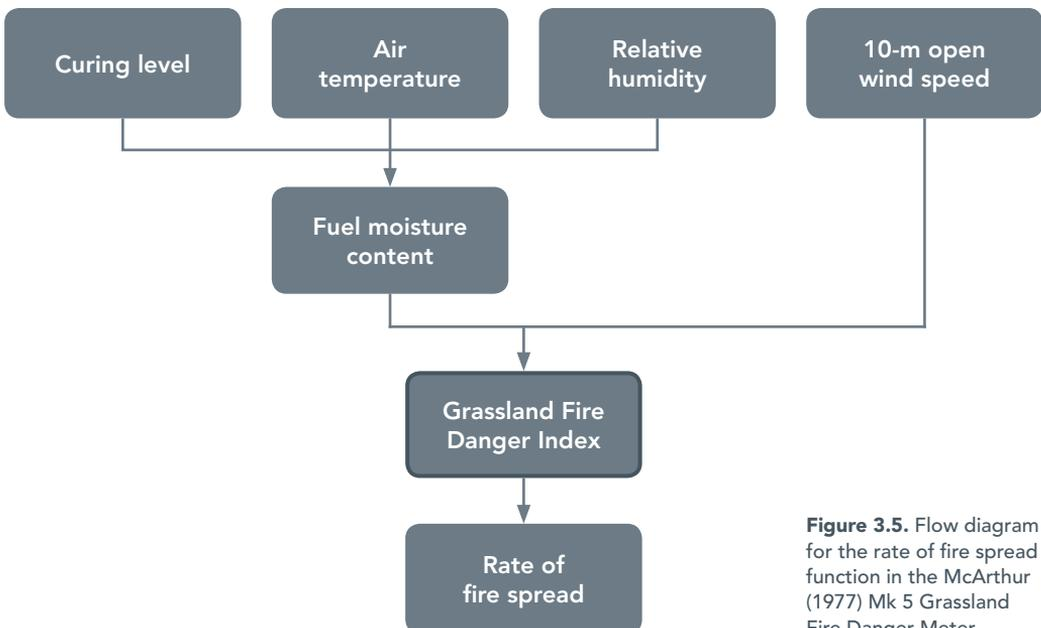
**Figure 3.5.** Flow diagram for the rate of fire spread function in the McArthur (1977) Mk 5 Grassland Fire Danger Meter.
