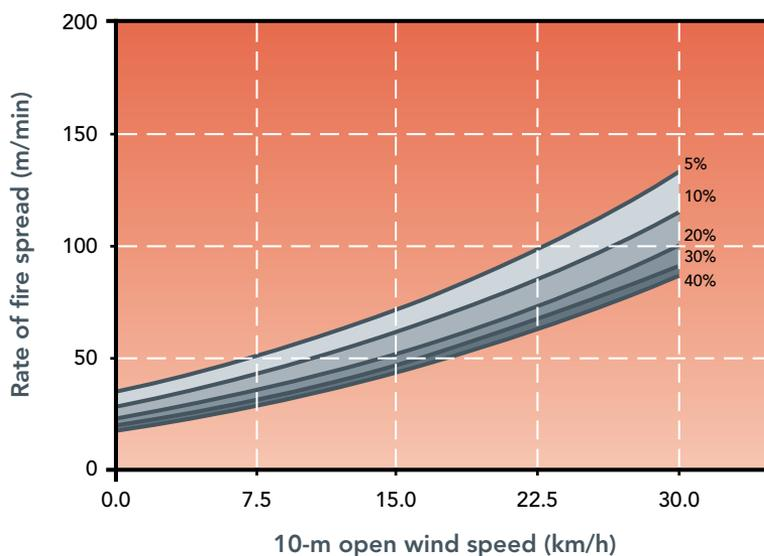
**Figure 3.12.** Prediction of rate of fire spread in spinifex according to the Griffin and Allan (1984) model as a function of 10-m open wind speed and fine fuel moisture content as expected to occur under prescribed burning conditions. The following conditions are assumed: air temperature 31°C, relative humidity 10%, cover 39%, bare ground 42% and patchiness 0.8. A wind adjustment factor of 0.7 was used to convert 10-m open into 2-m wind speeds.
