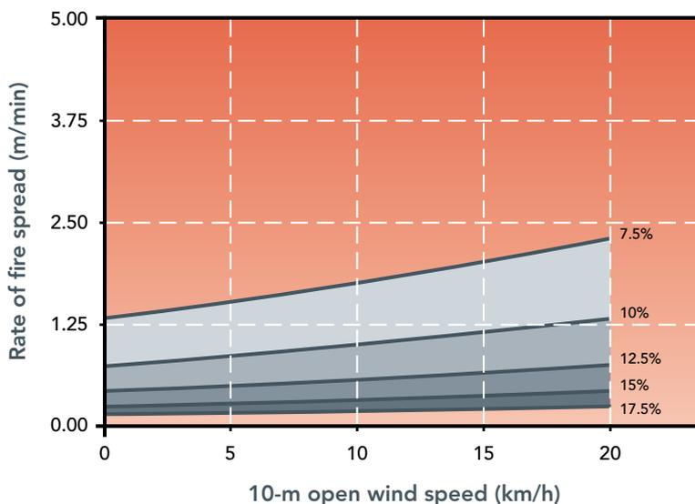
**Figure 5.4.** Prediction of rate of fire spread in eucalypt forests as a function of 10-m open wind speed and fine fuel moisture content as expected to occur under prescribed burning conditions as predicted by McArthur (1962) guide or model. A fuel load of 25 t/ha is assumed. Wind speed was converted from 10-m open to 1.5-m through Eq. 5.5.
