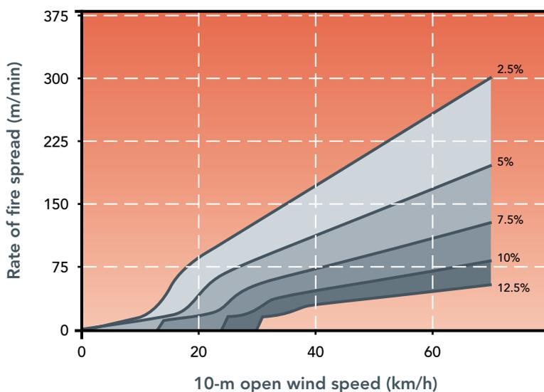
**Figure 4.19.** Prediction of surface and crown fire rate of spread in mallee-heath shrublands as a function of 10-m open wind speed and fine fuel moisture content as expected to occur under wildfire conditions according to the Cruz *et al.* (2013) model system. Simulation assumes a mallee overstorey cover of 33%.
