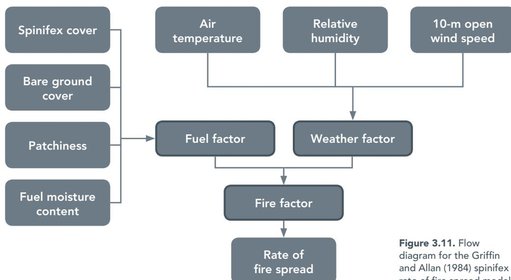
**Figure 3.11.** Flow diagram for the Griffin and Allan (1984) spinifex rate of fire spread model.
