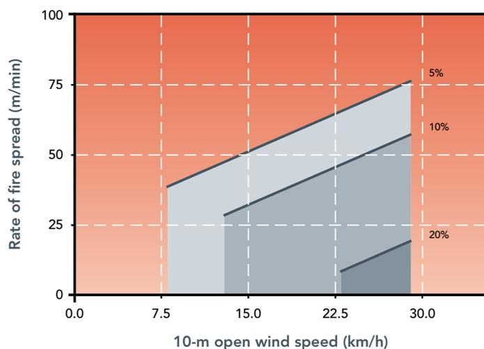
**Figure 3.18.** Prediction of rate of fire spread in spinifex according to the Burrows *et al.* (2009) model as a function of 10-m open wind speed and fine fuel moisture content as expected to occur under prescribed burning conditions. Fuel load of 7 t/ha is assumed. A wind adjustment factor of 0.7 was used to convert 10-m open into 2-m wind speeds.
