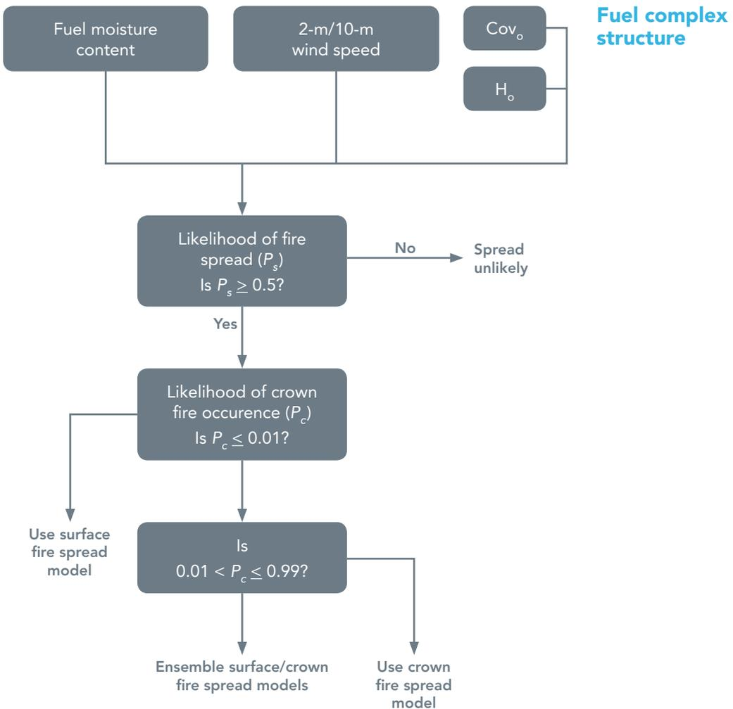
**Figure 4.18.** Flow diagram for the Cruz *et al.* (2013) model system to predict surface and crown fire rates of spread in semi-arid mallee-heath shrublands.
