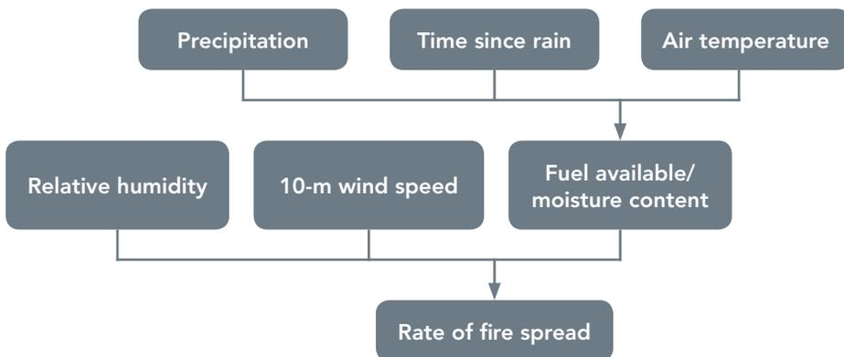
**Figure 7.4.** Flow diagram for Byrne (1980) model to predict the rate of spread of prescribed fires in slash pine plantations.
