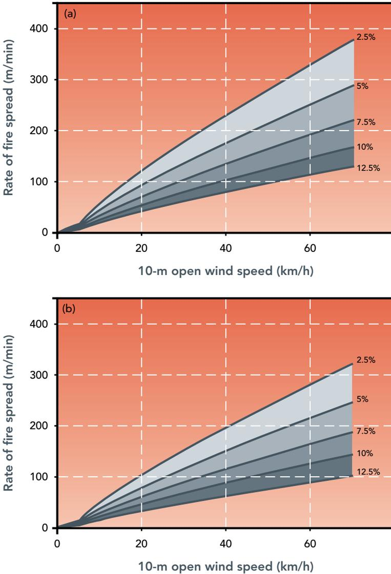
**Figure 3.10.** Prediction of grassfire rate of spread according to the CSIRO Grassland Fire Spread Meter (Cheney *et al.* 1998) for (a) undisturbed and (b) cut/grazed grasses as a function of 10-m open wind speed and fine fuel moisture content as expected to occur under wildfire conditions. 100% cured state is assumed.
