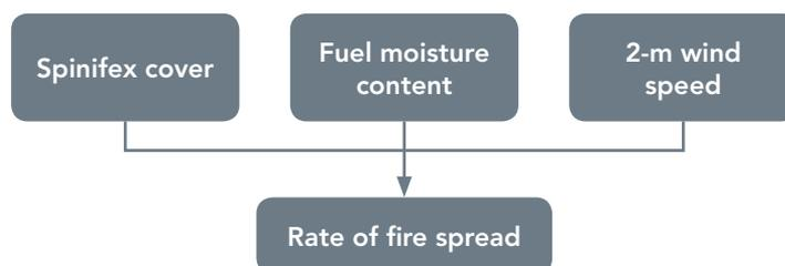
**Figure 3.13.** Flow diagram for the Burrows *et al.* (1991) spinifex rate of fire spread model.
