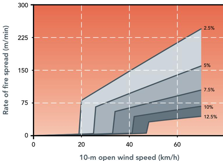
**Figure 7.10.** Prediction of rate of fire spread in pine plantations as a function of 10-m open wind speed and fine fuel moisture content as expected under wildfire conditions according to the Cruz *et al.* (2008) model system. A stand height of 14 m, a canopy base height of 6 m, and a canopy bulk density of 0.23 kg/m<sup>3</sup> are assumed.
