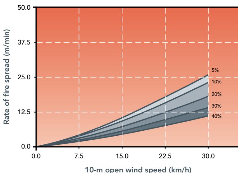
**Figure 4.5.** Prediction of rate of fire spread for buttongrass moorlands according to Marsden-Smedley and Catchpole (1995a) model as a function of 10-m open wind speed and fine fuel moistures content as expected to occur under prescribed burning conditions. A fuel age of 16 years is assumed. A wind adjustment factor of 0.67 was used to convert 10-m open into 2-m wind speeds.
