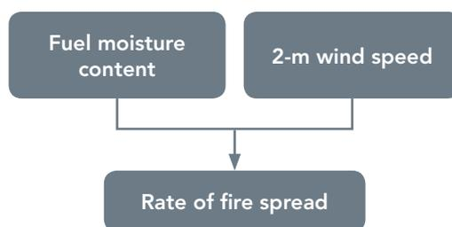
**Figure 4.11.** Flow diagram for the McCaw (1997) model for predicting the rate of fire spread in WA mallee-heath shrublands.
