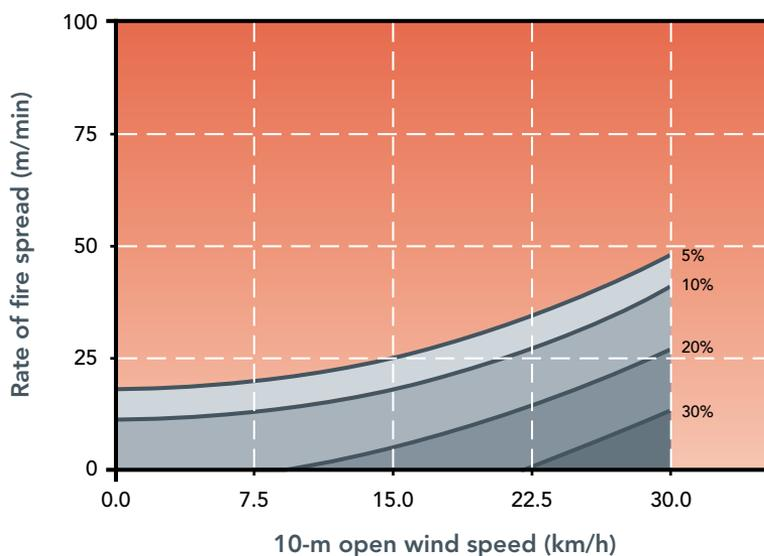
**Figure 3.14.** Prediction of rate of fire spread in spinifex according to the Burrows *et al.* (1991) model as a function of 10-m open wind speed and fine fuel moisture content as expected to occur under prescribed burning conditions. An air temperature of 31 °C, a spinifex cover of 40%, and bare ground of 45% are assumed. A wind adjustment factor of 0.7 was used to convert 10-m open into 2-m wind speeds.
