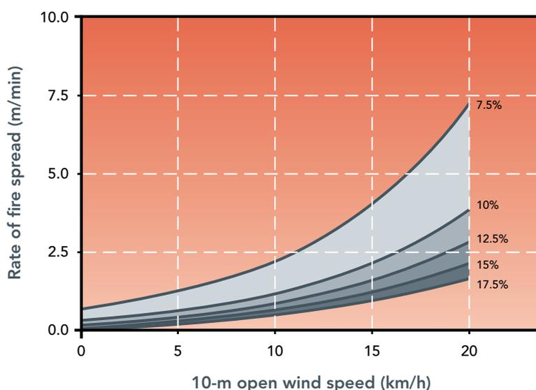
**Figure 5.7.** Prediction of rate of fire spread in jarrah forest as a function of 10-m open wind speed and fine fuel moisture content as expected to occur under prescribed burning conditions according to Sneeuwjagt and Peet (1985) Forest Fire Behaviour Tables of Western Australia model. A fuel load of 20 t/ha is assumed. A wind adjustment factor of 0.33 was used to convert 10-m open into 1.5-m wind speed (a wind ratio of 3:1, Beck 1995).
