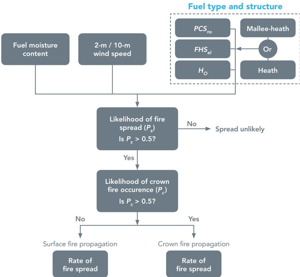
**Figure 4.14.** Flow diagram for the Cruz *et al.* (2010) model for predicting the rate of fire spread in SA mallee-heath shrublands.  $PCS_{ns}$  is the near surface fuel layer percent cover score,  $FHS_{el}$  is the elevated fuel hazard score and  $H_O$  is the height of the mallee overstorey layer.
