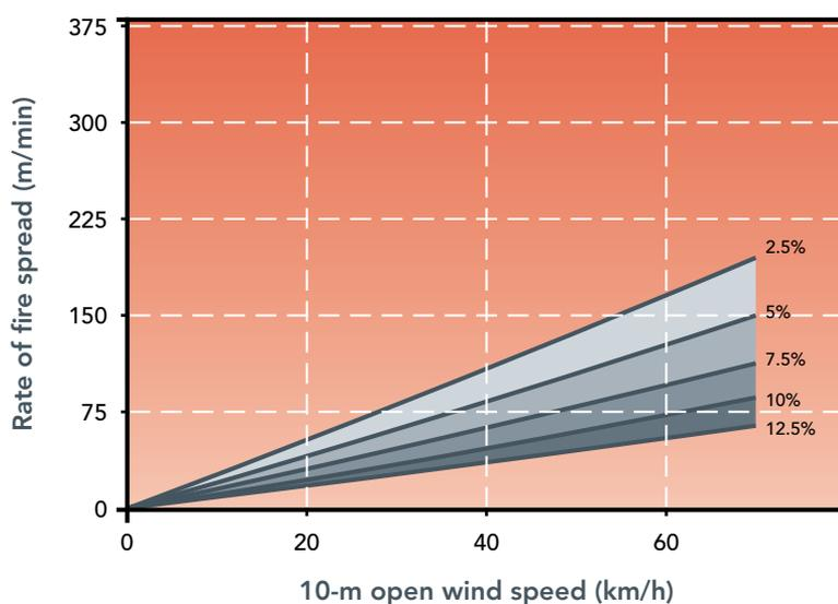
**Figure 4.12.** Prediction of rate of fire spread in mallee-heath shrublands as a function of 10-m open wind speed and fine fuel moisture content as expected to occur under wildfire conditions as predicted by the McCaw (1997) model. A wind adjustment factor of 0.67 was used to convert 10-m open into 2-m wind speeds.
