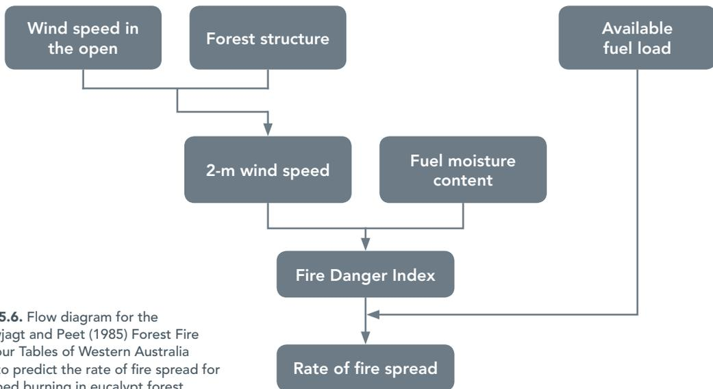
**Figure 5.6.** Flow diagram for the Sneeuwjagt and Peet (1985) Forest Fire Behaviour Tables of Western Australia model to predict the rate of fire spread for prescribed burning in eucalypt forest.
