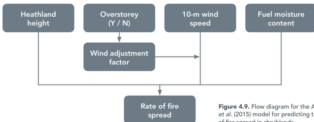
**Figure 4.9.** Flow diagram for the Anderson et al. (2015) model for predicting the rate of fire spread in shrublands.
