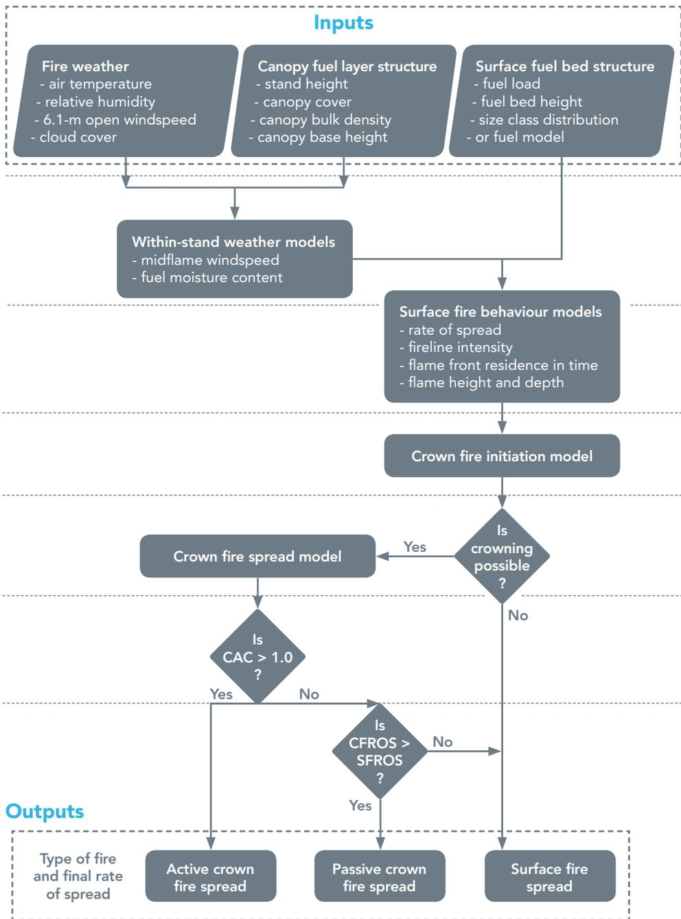
**Figure 7.9.** Flow diagram for the PPPY model system of Cruz *et al.* (2008) for predicting fire behaviour in pine plantations. CAC is the criteria for active crowning (Van Wagner 1977), CFROS is the crown fire rate of spread, and SFROS the surface fire rate of spread.
