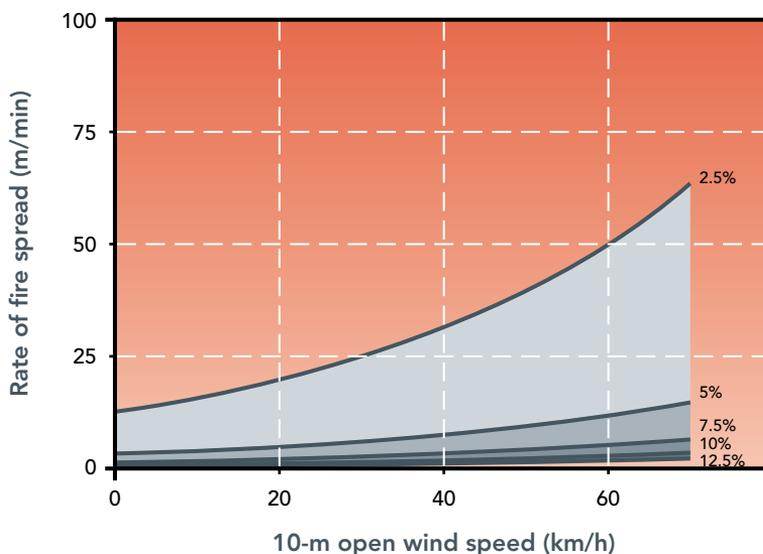
**Figure 5.13.** Prediction of rate of fire spread in dry sclerophyll eucalypt forests as a function of the 10-m open wind speed and fine fuel moistures content as expected to occur under wildfire conditions according to the McArthur (1967) Forest Fire Danger Meter. A fuel load of 25 t/ha and a D of 10 are assumed.
