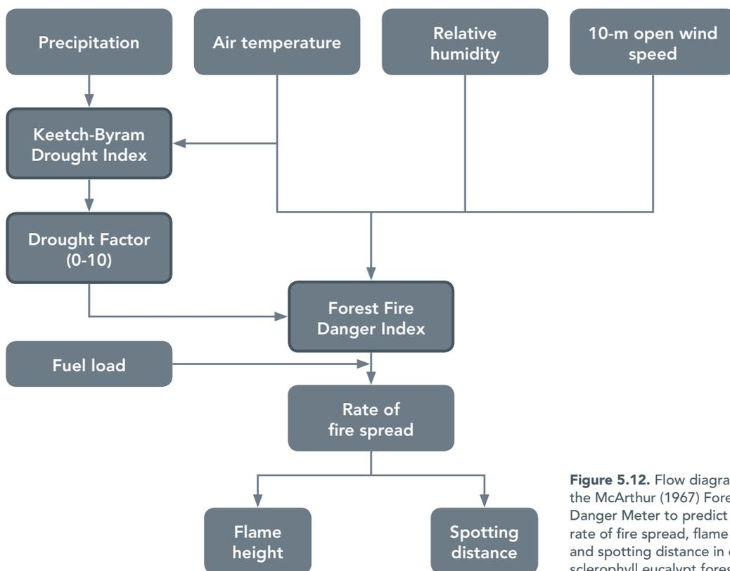
**Figure 5.12.** Flow diagram for the McArthur (1967) Forest Fire Danger Meter to predict the rate of fire spread, flame height and spotting distance in dry sclerophyll eucalypt forests.
