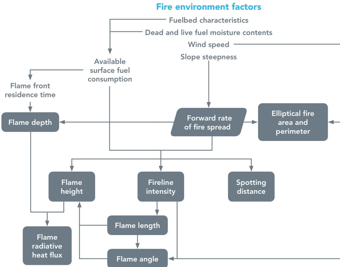
**Figure 2.1.** Flow chart illustrating the linkages that forward rate of fire spread has to the flame front dimensions and other fire behaviour characteristics (adapted from Cruz and Alexander 2013).
