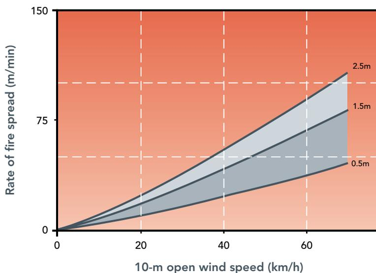
**Figure 4.8.** Prediction of rate of fire spread in shrublands as a function of 10-m open wind speed and fuel height as expected to occur under wildfire conditions according to the Catchpole *et al.* (1998) model. A wind adjustment factor of 0.67 was used to convert 10-m open into 2-m wind speeds.
