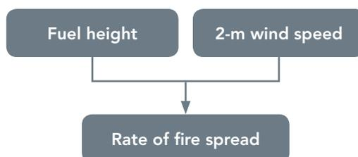
**Figure 4.7.** Flow diagram for the Catchpole *et al.* (1998) model for predicting the rate of fire spread in shrublands.
