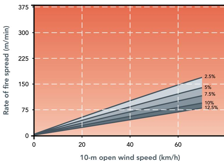
**Figure 4.10.** Prediction of rate of fire spread in shrublands as a function of 10-m open wind speed and fuel height as expected to occur under wildfire conditions according to Anderson *et al.* (2015) model. A fuel height of 1.5 m is assumed.
