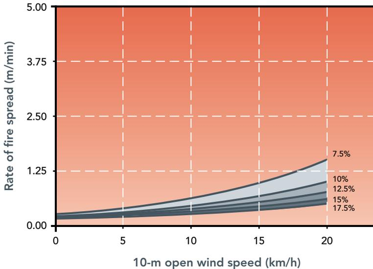
**Figure 6.2.** Rate of fire spread in karri forests as a function of 10-m open wind speed and fine fuel moistures content as expected to occur under prescribed burning conditions according to Sneeuwjagt and Peet (1985) Forest Fire Behaviour Tables of Western Australia model. Fuel load of 20 t/ha is assumed. A wind adjustment factor of 0.167 was used to convert 10-m open into 2-m wind speed (a wind ratio of 6:1, Beck 1995).
