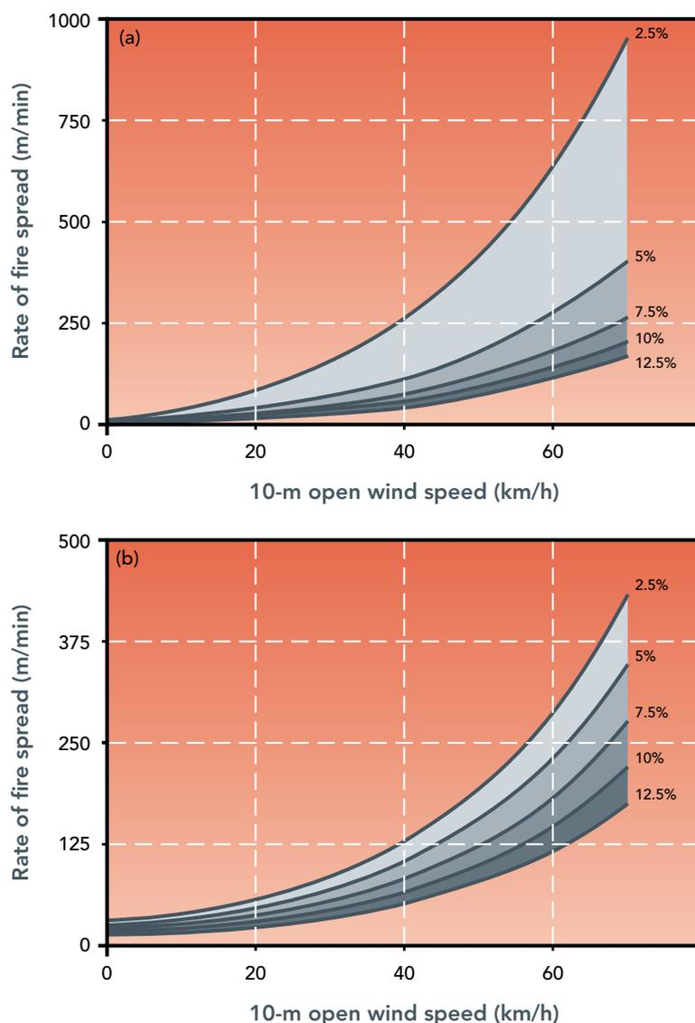
**Figure 3.6.** Prediction of grassfire rate of spread by (a) McArthur Mk 3/4 and (b) Mk 5 Grassland Fire Danger Meters as a function of 10-m open wind speed and fuel moisture content expected to occur under wildfire conditions. A curing level of 100% and a fuel load of 4.5 t/ha are assumed.
