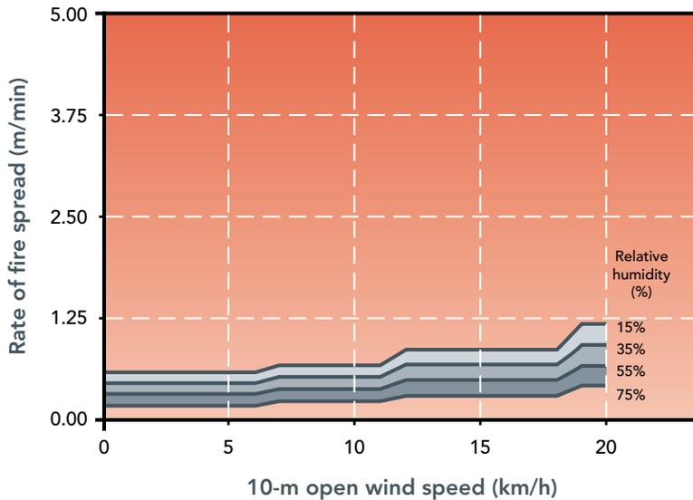
**Figure 7.5.** Prediction of rate of fire spread in slash pine plantations as a function of 10-m open wind speed and relative humidity as expected to occur under prescribed burning conditions according to the Byrne (1980) model.
