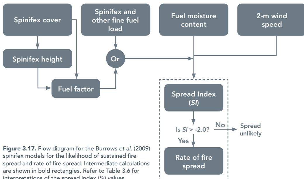
**Figure 3.17.** Flow diagram for the Burrows *et al.* (2009) spinifex models for the likelihood of sustained fire spread and rate of fire spread. Intermediate calculations are shown in bold rectangles. Refer to Table 3.6 for interpretations of the spread index (*SI*) values.
