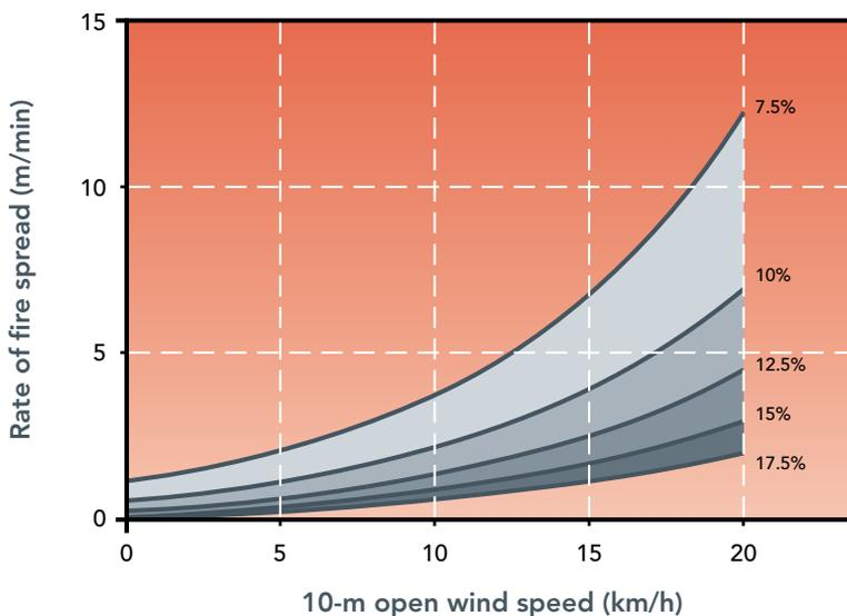
**Figure 7.7.** Predicted rate of fire spread in pine plantations as a function of 10-m open wind speed and fine fuel moisture content as expected to occur under prescribed burning conditions according to the Sneeuwjagt and Peet (1985) model. A fuel load of 15 t/ha is assumed. A wind adjustment factor of 0.33 was used to convert 10-m open into 1.5-m wind speed (a wind ratio of 3:1, Beck 1995).
