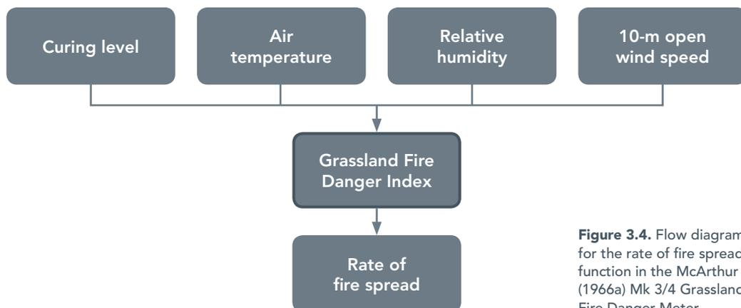
Figure 3.4. Flow diagram for the rate of fire spread function in the McArthur (1966a) Mk 3/4 Grassland Fire Danger Meter.
