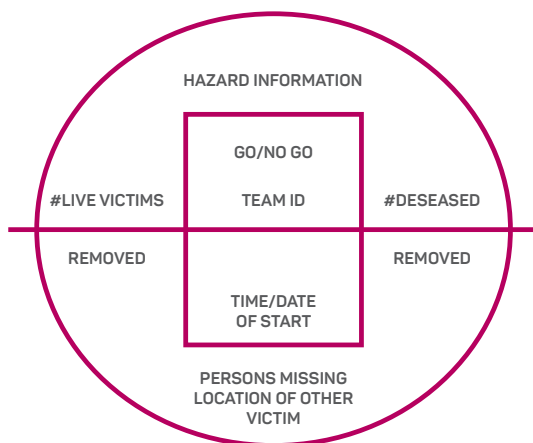
Figure 1: Former INSARAG Structural Marking (United Nations 2006).
